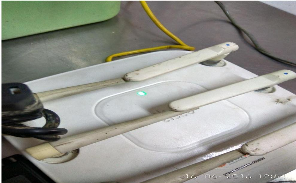
Gambar 3.12 Pengecekan Indikator Akses Point
